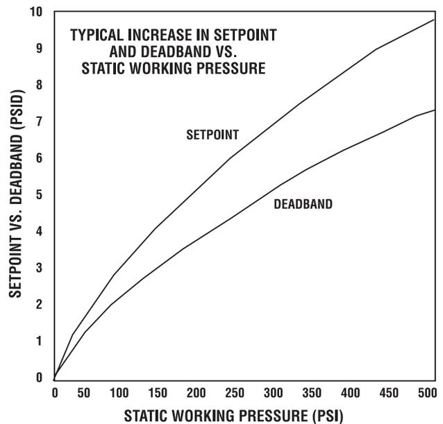
**Ex. 2. An L-Series**, single setpoint, 60 psid range, with a type “G” switch element, has a setpoint of 50 psid and a deadband of 7 psid at 200 psi static working pressure. If the static pressure could vary up to 300 psi, what change in setpoint and deadband could be expected?
