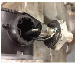
**Conclusion:** This test confirms that the DG25 enclosure is compliant with the IP-67 standard. The DG25 gauge can therefore be claimed as an IP-67 rated product.
