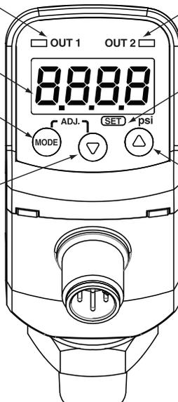
Pressing the **(MODE)** key for 3 seconds displays “\_\_\_”.” To return to measurement mode, the “\_\_\_” display will flash when 3 seconds have passed.
