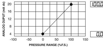
**Example 1)** Pressure range 0.00~1450 psi (0.0~100.0%F.S.) corresponding to analog output of 4~20mA dc is scaled to pressure range 0.00~1,423 psi (0.0~98.1%F.S.) corresponding to analog output 4~20mA dc.
