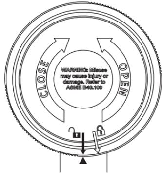
Remove cover by pulling straight back and replace AA alkaline batteries accordingly; ensure that the batteries are in the proper polarity position.
