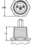
FLYING LEADS ELECTRICAL TERMINATION CONDUIT - 1/2 NPT MALE (C2), (C5)
