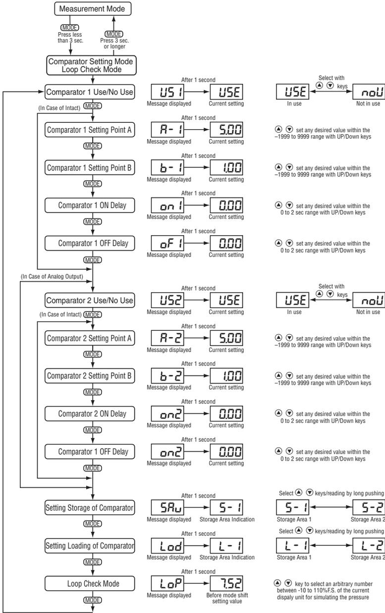
**Notes:** Values shown are from the example within the complete I&M manual. Changes made in the Setting Mode are saved by returning to Measurement Mode before powering off the unit.
