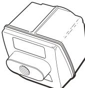
AM2-RT1 and RT2 modules are RTD temperature measurement modules compatible with Pt100, Pt1000, Ni120, Cu10, and up to six user programmable resistance curves. Measurements can be displayed in degrees Fahrenheit, Celsius, Kelvin, Rankin or ohms. The setup menu allows the operator to choose configurations for 2, 3 or 4 wire RTD probes. In addition, the setup menu also allows selection of 1, 0.1, 0.01 or 0.001 decimals of resolution. Accuracy specifications are detailed in the data sheet.
