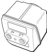
AM2-2 are high pressure measurement devices. They are single-port modules based on sensors capable of measuring gauge, absolute, compound or vacuum with ranges spanning from vacuum to 5 psi to 10,000 psi. All wetted parts are 316 stainless steel (except for 10k psi module which has 17-4ph stainless steel) and are intended for use with any pressure medium compatible with stainless steel.
