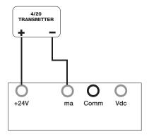
4/20 TRANSMITTER HOOK UP USING, EXTERNAL SUPPLY
