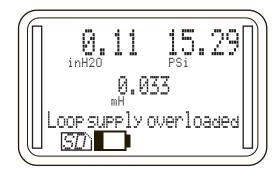
Remove the overload from test circuit and enable the 24 VDC power supply via MENU commands. (See section 14k)
