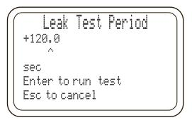
Press ENTER to immediately begin Leak Decay Test. When test is complete the decay value will be displayed in the unit of measure selected previously. Pressure decrease will display as a positive value, pressure increase will display as a negative value.
