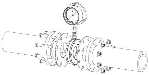
(Exploded View) Gaskets, nuts and bolts provided by USER
