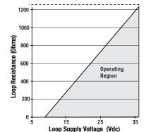
V<sub>MIN</sub> = 9V + (0.022\*A x R<sub>L00P</sub>) (\*includes a 10% safety factor)  $R_{LOOP} = R_{SENSE} + R_{WIRING}$ RLOOP = Loop Resistance (Ohms) Rsense = Sense Resistance (Ohms)
