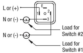
View of plug after removing the socket
