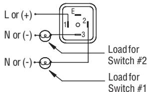
View of plug after removing the socket
