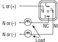
View of plug after removing the socket
