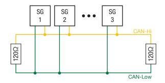
Figure 1: Linear CAN bus topology with terminating resistors [1]
