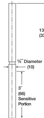
13" plain bulb for applications used in open tanks where pressures and velocities are negligible
