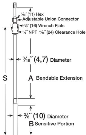
The bendable extensions with union connections. B01 [12" bendable extension] is the standard Duratemp bulb style and is suitable for a variety of insertion lengths and lagging requirements. B17 is a 18" bendable extension, B18 is a 24" bendable extension.
