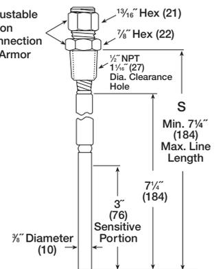
The compression fitting fastens anywhere along the armored line. This Bulb Style is well suited for insertion requirements in excess of 13 1/2". The B08 style is not a pressure tight connection. A thermowell is recommended for this style and for all bulb styles.
