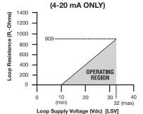
To determine minimum loop supply voltage:
