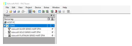
Select the DTM and connect to start the communication with the device. Double clicking the connected DTM will open the Online-parametrization window (Offline, if device is not connected).
