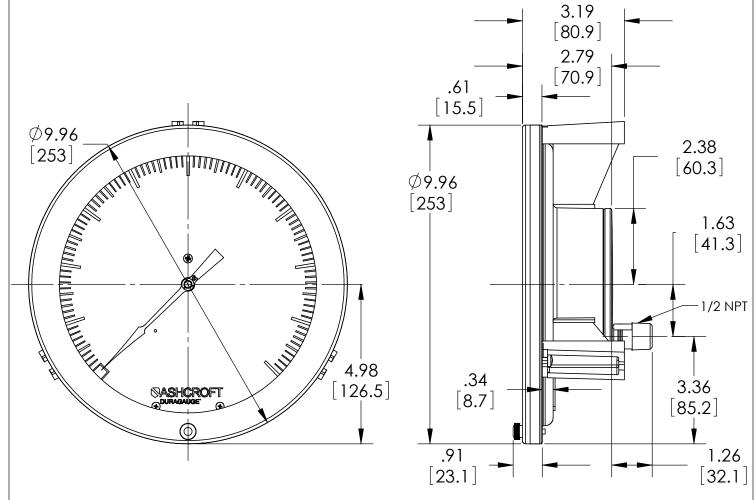
Note: 3 Mounting studs threaded equally spaced on a 9.625" [244] Bolt Circle.
