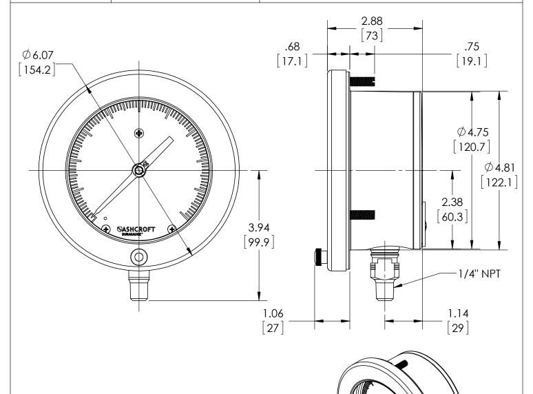
Note: 3 Mounting studs threaded equally spaced on a 5.375" [137] Bolt Circle.
