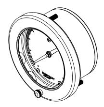
Note: 3 Mounting studs threaded equally spaced on a 5.375" [137] Bolt Circle.
