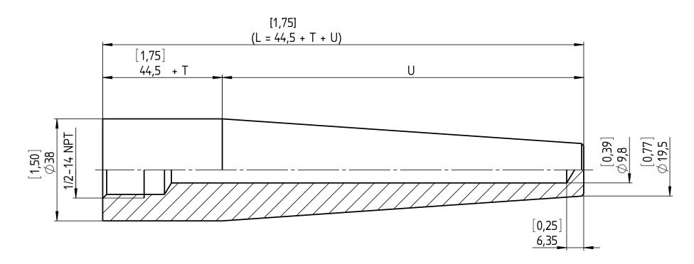
U-LENGTH (SPECIFY BY CUSTOMER) T-LENGTH (SPECIFY BY CUSTOMER) FOR L-LENGTH ≥ 1300 MM THE THERMOWELL WILL BE MANUFACTURED IN PIECES!
