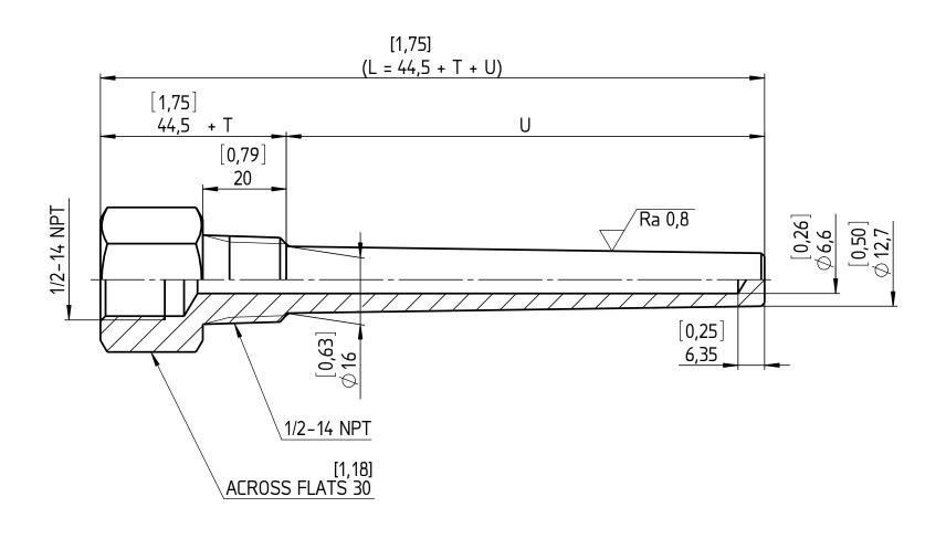
U-LENGTH (SPECIFY BY CUSTOMER) T-LENGTH (SPECIFY BY CUSTOMER) FOR L-LENGTH ≥ 1300 MM THE THERMOWELL WILL BE MANUFACTURED IN PIECES!
