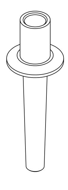
OPTIONAL CAP AND CHAIN U-LENGTH (SPECIFY BY CUSTOMER) T-LENGTH (SPECIFY BY CUSTOMER) FOR L-LENGTH ≥ 1300 MM THE THERMOWELL WILL BE MANUFACTURED IN PIECES!
