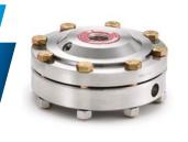
The Ashcroft<sup>®</sup> 740 and 741 high-displacement diaphragm seals or isolation devices are used with low-ranged instruments or high static pressure dp gauges with low differential pressure. Used to ensure material compatibility, they are also applied when process media exhibits high temperature, pulsation or the potential to clog an instrument connection. An ideal product for satisfying low pressure measurement needs.
