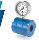
The Ashcroft® 82 isolation ring or isolation device is threaded in-line with process piping. Used on threaded piping systems for protection of measuring instruments. The "ring" design eliminates process accumulation, assuring accurate pressure readings.
