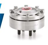
The Ashcroft<sup>®</sup> 702 and 703 high-displacement diaphragm seals or isolation devices are used with low pressure or differential pressure gauges with low differential pressure and elevated static pressure. Used to ensure material compatibility, they are also applied when process media exhibits high temperature, pulsation or the potential to clog an instrument connection. An ideal product for satisfying low pressure measurement needs.
