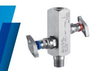
The Ashcroft<sup>®</sup> multiport valve-V02 is designed to mount directly to the instrument for the purpose of isolating up to three instruments simultaneously during process shut downs and maintenance.
