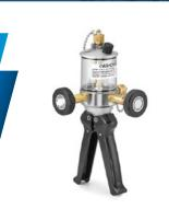
The QTHP is a portable hydraulic hand operated pump capable of generating up to 5,000 psi (345 bar) using liquid media including water, alcohol, oils and hydraulic fluids.
