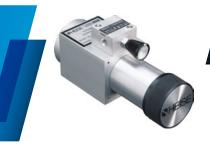
The Ashcroft<sup>®</sup> AVC-1000 and AVC-3000 pressure volume controllers provide a means to precisely set pressures within a closed pneumatic system. Providing quick-and-easy operation, models are paired with test gauges, creating a reliable standard for calibration and test purposes.
