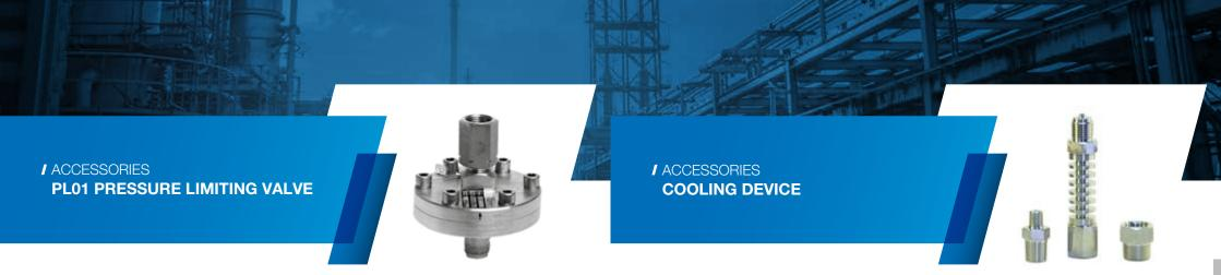
The Ashcroft® pressure limiting valve-PL01 automatically closes when set pressure is realized. When the valve closes, the instrument assembly is isolated and protected during pressure excursion beyond the full scale range of the instrument.
