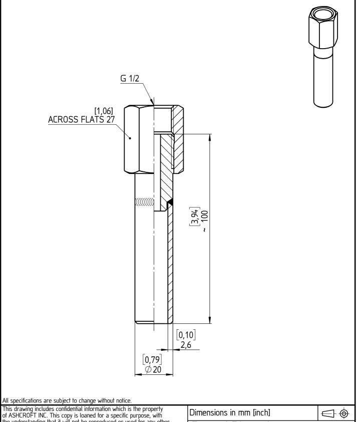
This drawing includes confidential information which is the property of ASHCROFT INC. This copy is loaned for a specific purpose, with the understanding that it will not be reproduced or used for any other General Dimension purpose or disclosed to others, and it will be returned on demand. Name Date Pipe Connector Drawn 23.05.17 J. Krott Checked 23.05.17 Welding connection, straight pipe, G 1/2f swivel DWG. NO. **SASHCROFT** A 076 I 8-PIPE-00-PC-A-81-100 Description Date Na. Rev.
