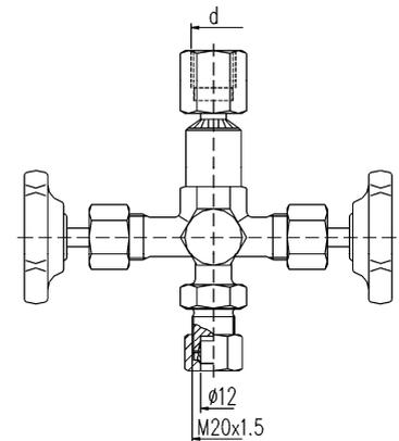
tube fitting O. D. 12 mm line S
