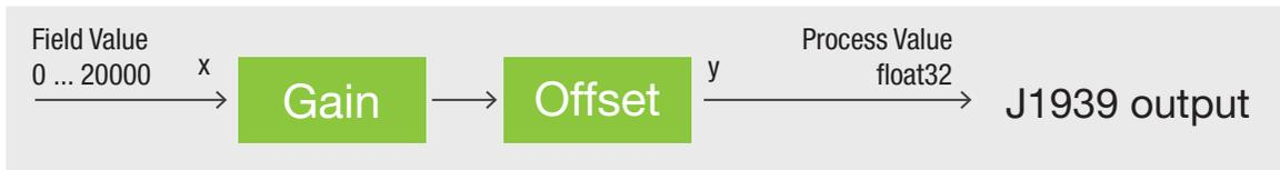
The transducer's nominal measuring range corresponds to the internal Field Value range of [0...20000]. Using the *gain* and *offset* parameters, these internal values are being scaled according to the following formula:
