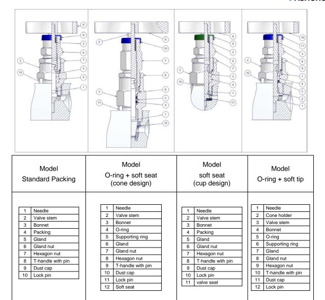
Note: Spindle seals, packing and O-ring can be used with the various valve seats combined may occur.
