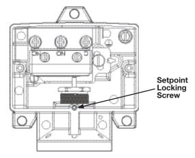
After installation of the control replace cover to insure electrical safety and to protect internal parts from the environment.
