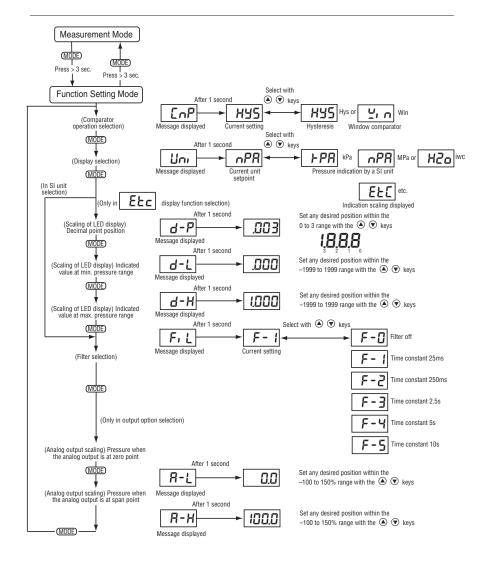
**Caution:** Editing the setting value in function setting mode resets all of the setting values including the switch. Please note that when the reset setting values are out of the display range, they will be adjusted to an upper or lower limit value that can be processed internally.
