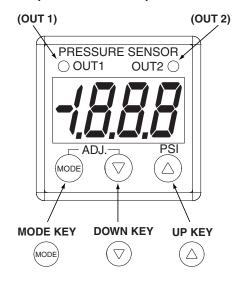
Pressing the (MODE) key for 3 seconds displays "---". To return to measurement mode from each setting mode, the "---" display will flash when 3 seconds have passed.
