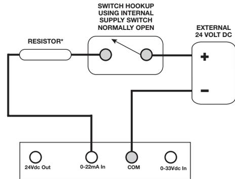
\*Resistor should be sized to allow current as follows:
