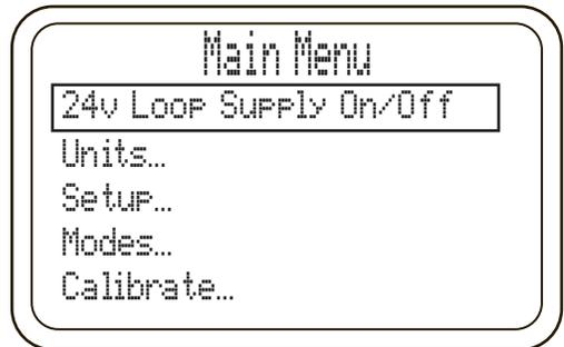
HHC will return to Measurement Mode and "24v" is shown on center bottom of display to indicate power supply is activated.
