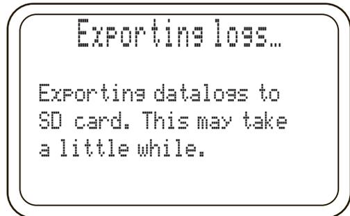
Datalogs will appear in a folder on the SD card labeled DATALOGS.
