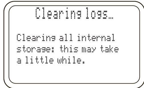
When the operation is complete the HHC will return to Measurement Mode.
