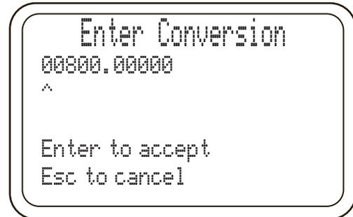
Press left and RIGHT ARROWS to position cursor beneath desired numeric character.
