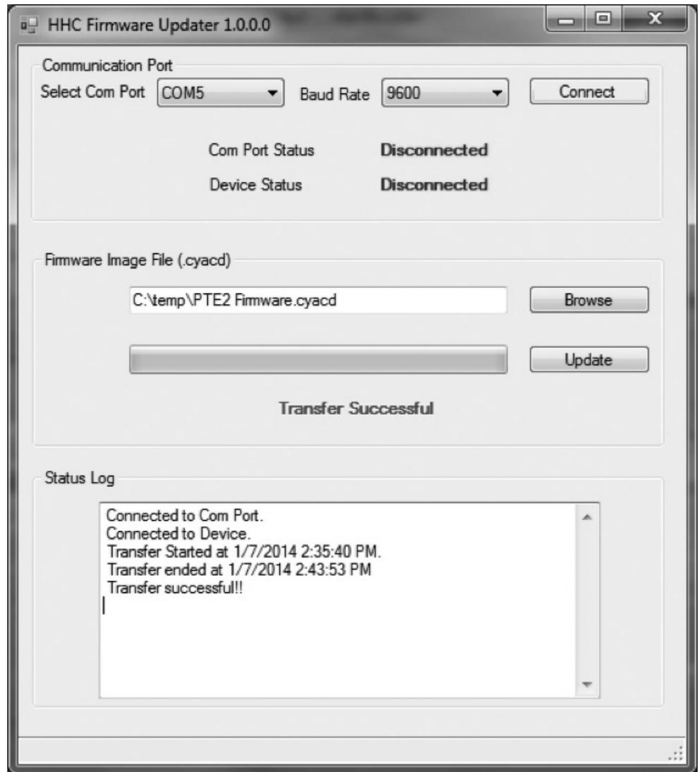
When the "Transfer Successful" message is displayed the process has completed. You can verify the update was successful by powering on the HHC base unit and noting the new firmware revision number displayed during boot up and in the "about this HHC..." MENU under Setup/System.
