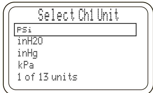
Press Enter to select unit and exit to Measurement Mode.
