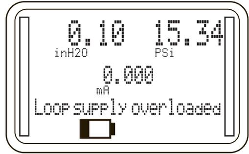
Remove the excessive load from the circuit and attempt to activate the 24v loop power supply via the MENU as described above.
