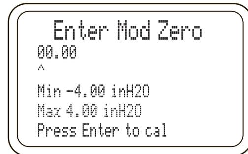
Note: Min and Max allowable limits for all calibration pressure values will be displayed below the target cardinal value. If the pressure standard does not achieve exactly the target
