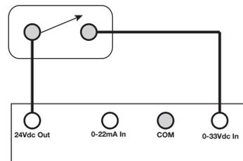
EXTERNAL 24 VDC SUPPLY SWITCH HOOKUP USING INTERNAL SUPPLY SWITCH NORMALLY OPEN
