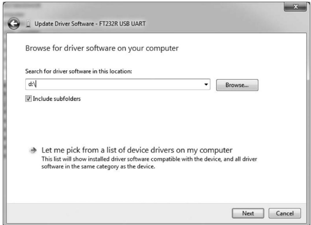
Windows will install the driver. Once complete an HHC will enumerate as a Communications Port on this computer. The driver installation should not have to be performed again.
