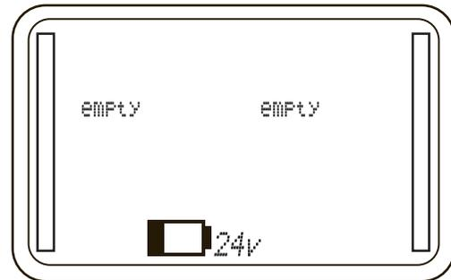
If the power supply has been overloaded and a warning message shows on the display (supply current is specified at 35ma and will overload at approximately 54-55ma)
