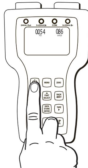
When powering on, the LCD display will briefly indicate the calibrator model number, serial number, owner information and whether it is an intrinsically safe or not intrinsically safe model. If pressure or temperature modules are installed, serial number,
