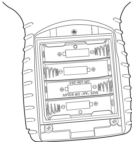
4. Install four new AA Alkaline batteries. (Only Duracell Alkaline part number MN1500 for I.S. units.) Observe polarity markings to install batteries correctly. Never mix old and new batteries.
