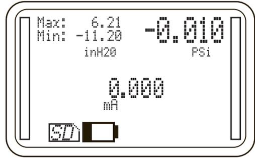
To clear active Min/Max measurements press the ZERO key.
