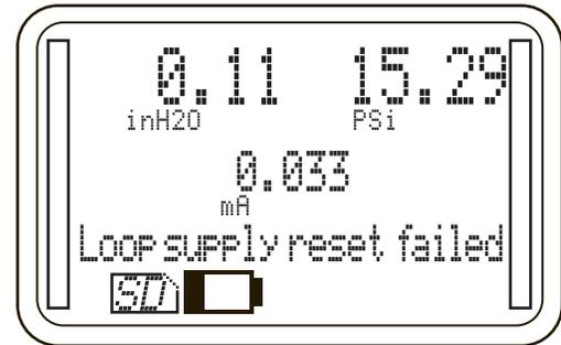
Note: A direct short between 24Vdc out and COM terminals will cause complete shut down of the base unit. Remove shorted leads and power the HHC on with the power key. Base unit will not be damaged, however warning messages will not be displayed.
