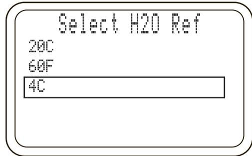
Press ENTER to select temperature and exit to Measurement Mode.
