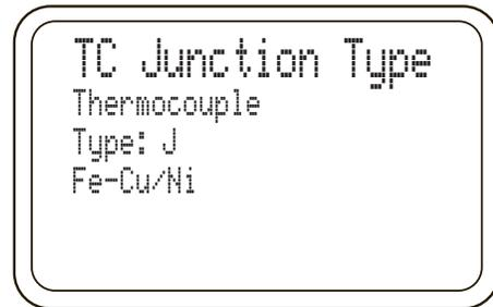
Note: By selecting the thermocouple type the PTE-2 will access the factory programmed coefficients in the module which will allow the PTE-2 to display in a unit of temperature
