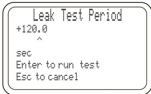
Press ENTER to immediately begin Leak Decay Test.
