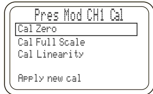
NOTE: Cal Zero function must be performed prior to proceeding to Cal Full Scale; Cal Zero & Cal Full Scale functions must be performed prior to proceeding to Cal Linearity. The "Cal Full Scale" & the "Cal Linearity" keys are activated only when this sequence is observed. The "Apply New Cal" function can be performed after each individual calibration steps (Zero, Full Scale, Linearity) was completed.
