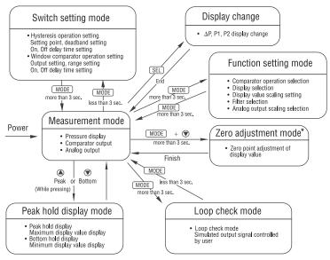
\*Note: Zero Adjustment, select P1 and P2 respectively and then use Zero Adjustment, will not function in DP mode.
