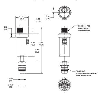
MVT - 18 UNF (compatible with 1/4 VCR®) Male Flow Through
