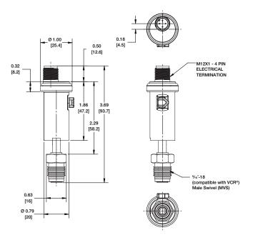
MVT - %16-18 UNF (compatible with 1/4 VCR®) Male Flow Through
