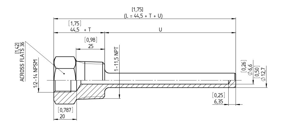
U-LENGTH (SPECIFY BY CUSTOMER) T-LENGTH (SPECIFY BY CUSTOMER) FOR L-LENGTH ≥ 1300 MM THE THERMOWELL WILL BE MANUFACTURED IN PIECES!
