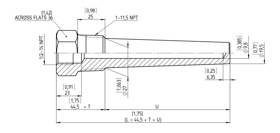
U-LENGTH (SPECIFY BY CUSTOMER) T-LENGTH (SPECIFY BY CUSTOMER) FOR L-LENGTH ≥ 1300 MM THE THERMOWELL WILL BE MANUFACTURED IN PIECES!
