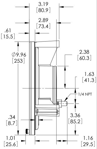
Note: 3 Mounting studs threaded equally spaced on a 9.625" [244] Bolt Circle.
