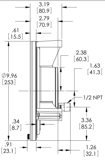
Note: 3 Mounting studs threaded equally spaced on a 9.625" [244] Bolt Circle.
