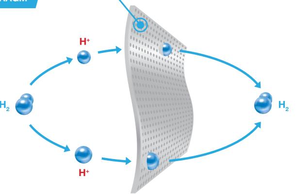
One way to reduce hydrogen permeation is to use a material with a dense lattice structure such as 316L stainless steel or variants of 316 stainless steel with a large membrane thickness. Another solution is to provide the membrane with a very thin gold layer. The gold layer has a very dense lattice structure that increases the membrane's resistance to hydrogen penetration.
